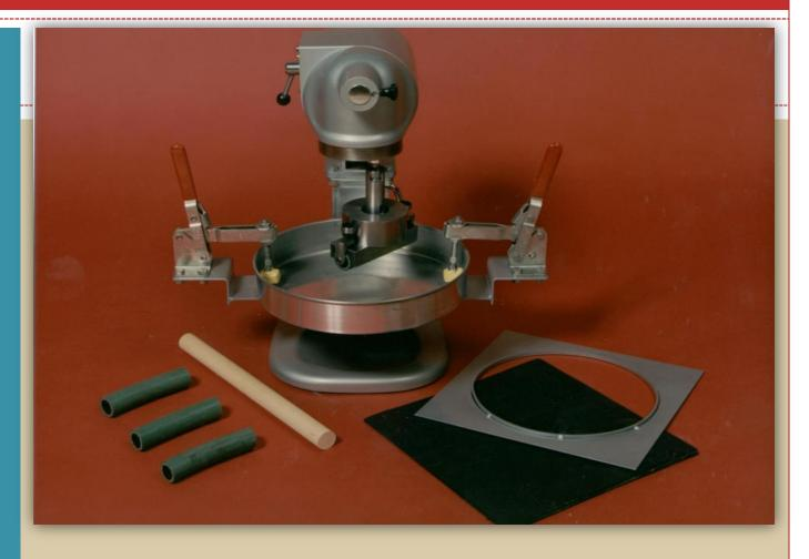
**Wet Track Abrasion Test Machine**
