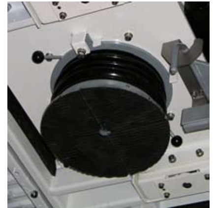
The four-split loading plate allows good contact to the surface and accurate measuring.
