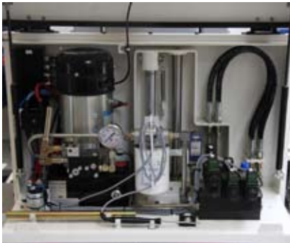
The weight system is 100% hydraulically operated. This gives good and stable control.
