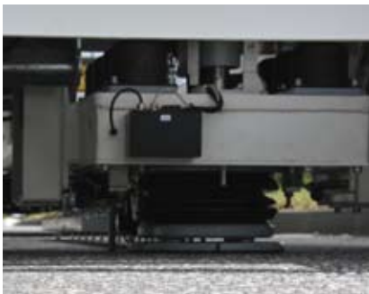
The four-split loading plate allows good contact to the surface and accurate measuring.
