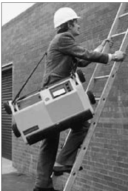
Weighing only 18 pounds the Dec Scanner can be easily carried up a ladder
